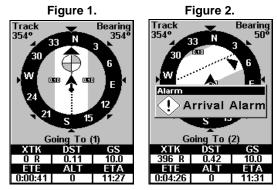
Fig. 1 shows the Navigation Page at the start of a route, heading straight for the first waypoint (Wpt 1). In Fig. 2, the traveler has arrived at Wpt 1; the arrival alarm has been triggered and the bearing arrow on the compass rose has turned to point toward Wpt 2, off to the northeast.
